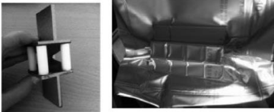
Figure 1. AE2 sample with PTFE wedges (left); sealed package of AE2 samples for aging without oxygen (right).
