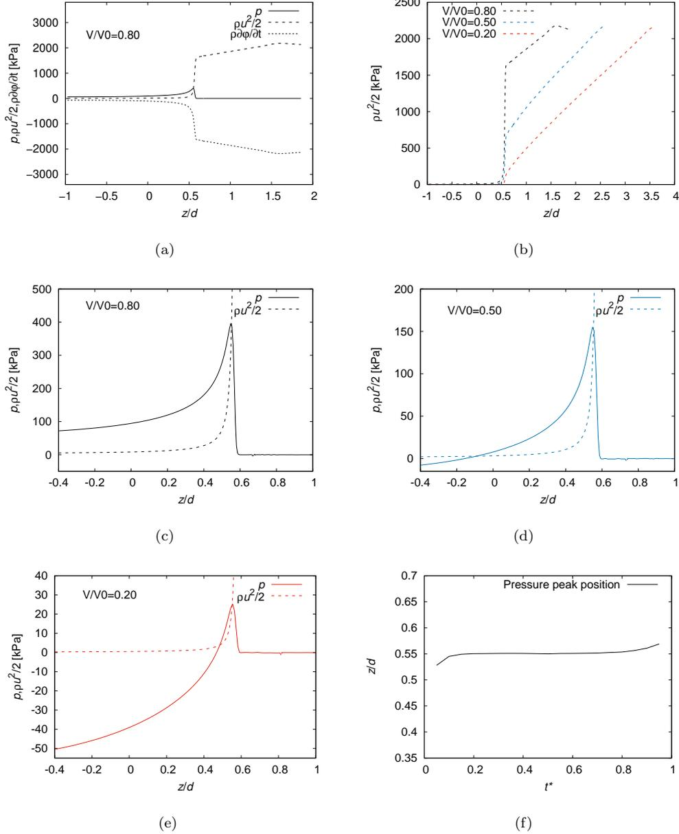
Figure 7: Wedge: pressure details. a) Comparison between the pressure, the non-linear term and the unsteady term of the Bernoulli's equation at  $V/V_0 = 0.80$ . b) Non-linear term of the Bernoulli's equation at three different time steps. c-e) Close-up view of the pressure (solid line) and the non-linear term of the Bernoulli's equation (dashed line) at  $V/V_0$  :  $c = 0.80, d = 0.50, e = 0.20$ . f) Time history of the pressure peak position scaled with the current depth.
