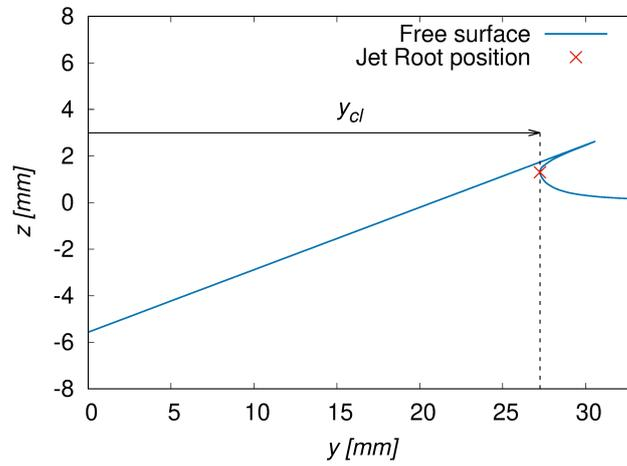
Figure 14: Definition of the contact line
