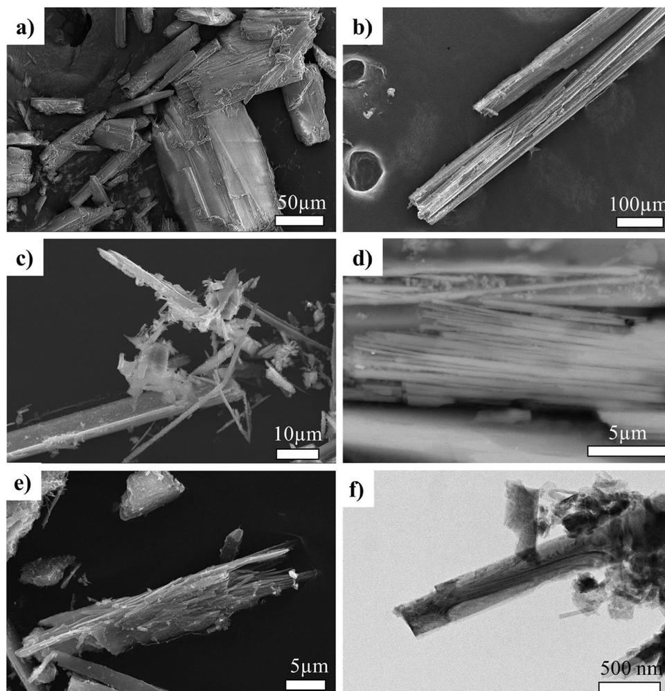
**Figure 3.** SEM and TEM images of tremolite find in the sample SMA1971-214. (a) SEM images of columnar aggregates with elongated prismatic habit. (b) SEM image of fibres bundles. (c) Tremolite asbestos fibres, (d) SEM images of tremolite fibres bundles. (e) SEM images of bundle of thin tremolite fibres, (f) TEM images of the tremolite single fibre and encrusting lizardite.
