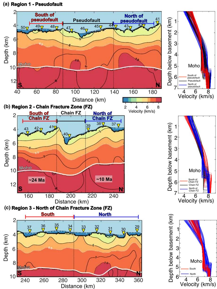
**Figure 9.** Close-up velocity models for (a) Region 1—the pseudofault, (b) Region 2—the Chain Fracture Zone, and (c) Region 3—the zone north of the Chain FZ. The location of each of the regions is shown in the 2-D profile in Figure 5b. Within each panel we identify zones from which we extract 1-D velocity functions spaced at 800 m for comparison. The extracted 1-D velocity functions are shown in the right of the corresponding region. The remaining elements are the same as in Figure 5.
