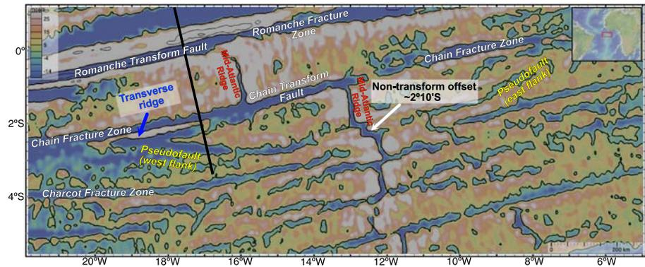
**Figure 7.** Global free-air anomaly map (Sandwell et al., 2014) for the equatorial Atlantic region with the interpretation of the main tectonic features indicated. The black line shows the location of the OBS line collected during the ILAB-SPARC cruise. The map is made using GeoMapApp (Ryan et al., 2009).
