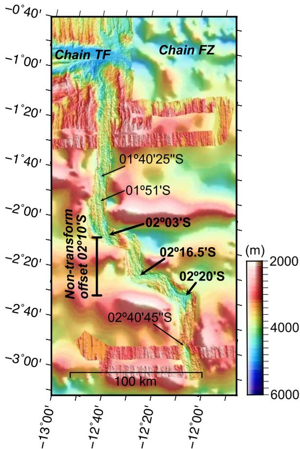
**Figure 6.** Bathymetry map of the first-order tectonic segment extending south of the Chain TF. The background is represented by GEBCO data on which high-resolution bathymetry data collected during the LITHOS experiment (Grevemeyer et al., 2019) are superimposed. The arrows indicate higher-order (second- and potentially third-order) discontinuities we identified in the seafloor.
