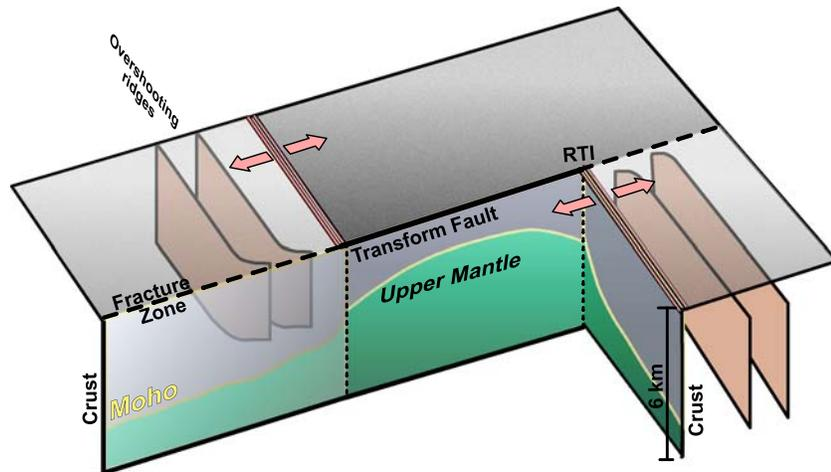
**Figure 13.** Schematic diagram that depicts lateral dike propagation as our preferred mechanism behind the presence of thicker crust within the fracture zone domain when compared with the transform fault domain.
