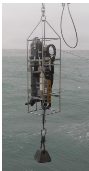
Figure 30 : Hydrological station. The SBE 19 sensor and the Niskin Bottle
