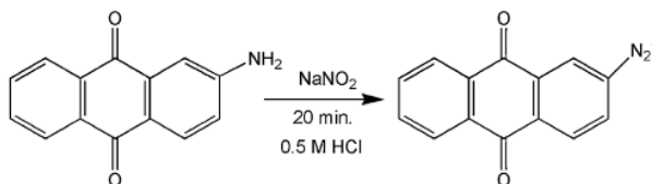
Scheme 1 : Diazotization of 2-aminoanthraquinone with NaNO 2 in 0.5 M HCl
