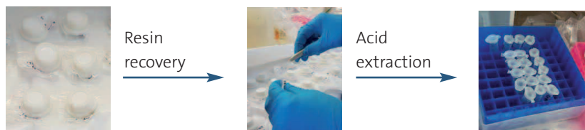
Image 13. General flow chart of DGT dismantling and extraction pre-analysis (Source: IFREMER).
