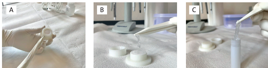
Image 12. (A) DGT opening; (B) Chelex-100 peel off; (C) Chelex-100 being placed in a sample tube (Source: UNICA).
