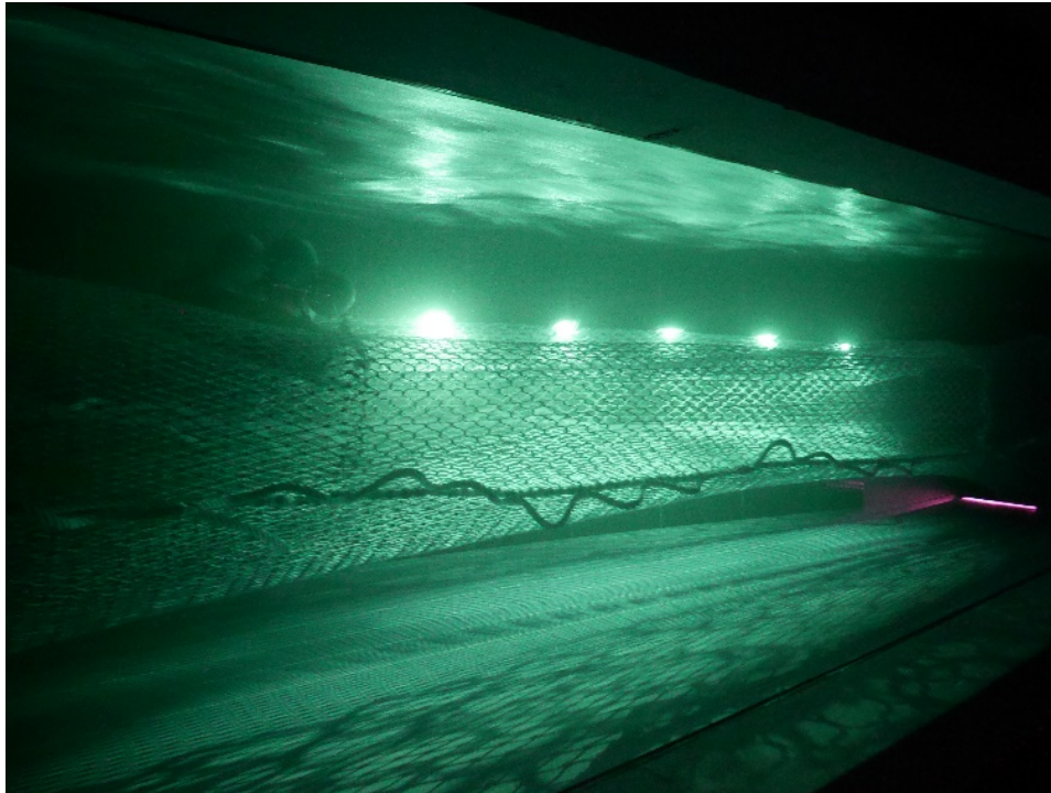
Figure 2: Preliminary trials with SafetyNet lamps in Lorient flume tank
