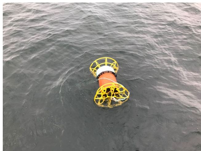
Figure 35: Spool at surface after being released from depth acoustically.
