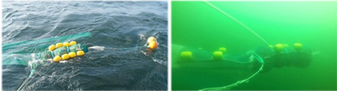
Figure 9: Codend floats and codend buoy. Right: Additional floats in front of the codend
