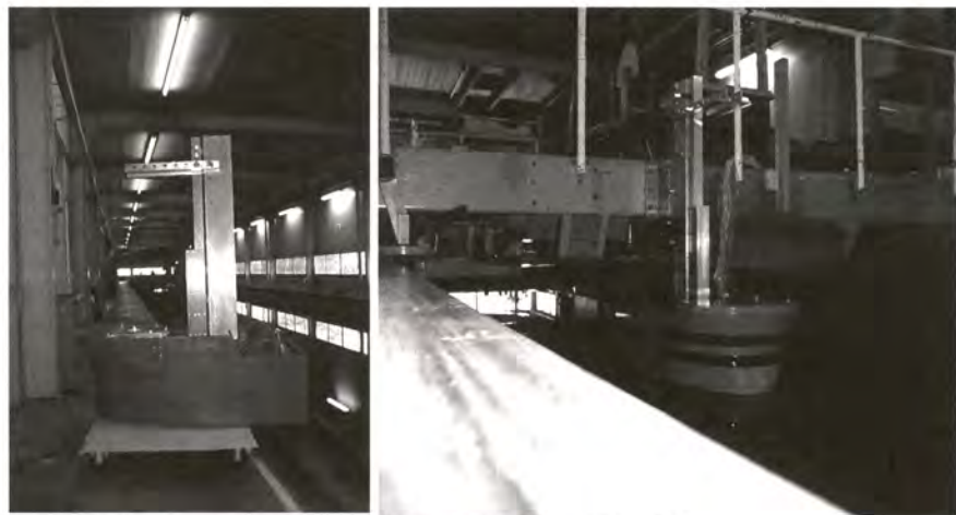
Fig. 4. The bow model (without seals and, in the tank, with seals)
