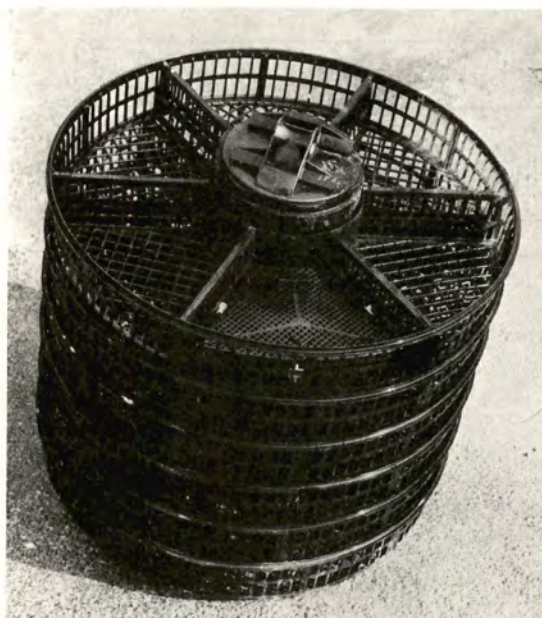
FIGURE 4 : Sample of creel used in suspended culture. The creel is open to show the upper tray. The compartments of the tray are filled with screened cells in which the spat is laid. One of these cells can be seen in the figure.
