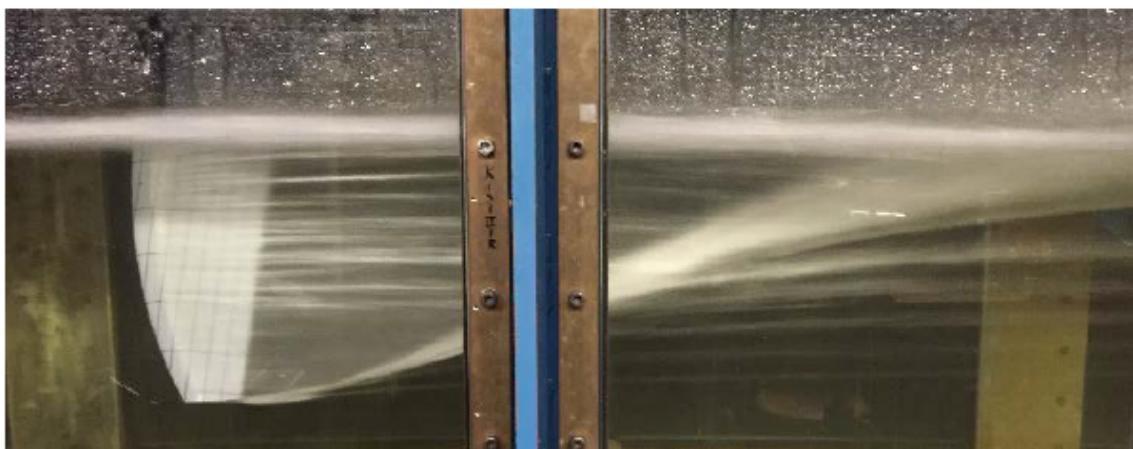
FIGURE 1.16 – Ventilation phenomenon on a surface piercing A-class catamaran hydrofoil [1]
