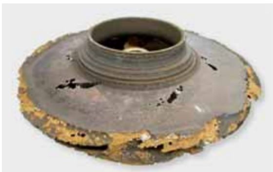
(a) Pump rotor destroyed by cavitation erosion.
