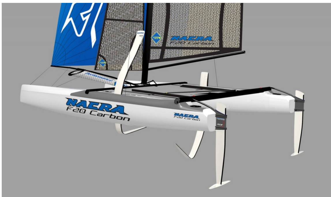
FIGURE 1.7 – Racing catamaran Nacra F20 FCS equipped with L-Foil, [107]
