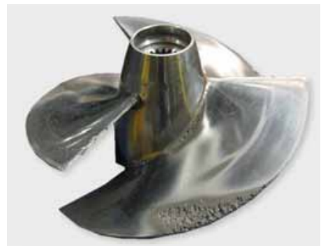
(b) propeller blade destroyed by cavitation erosion.
