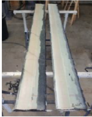
FIGURE 2.33 – Hydrofoils after demolding
