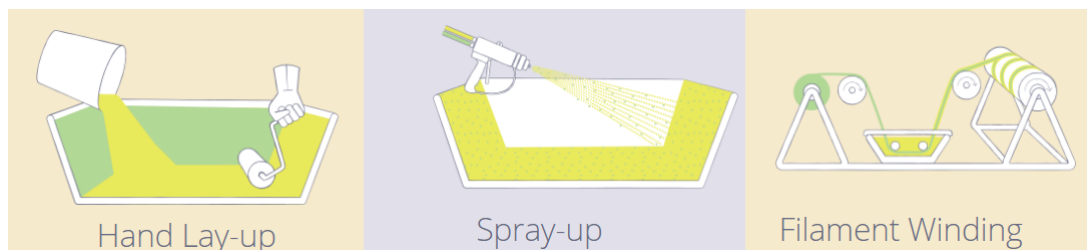
FIGURE 1.28 – Open molding processes
