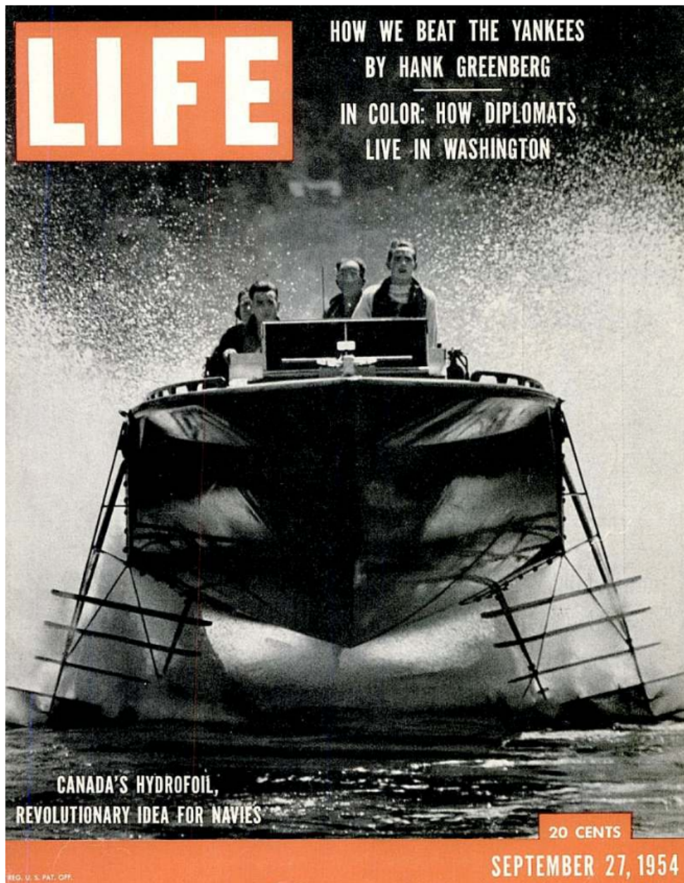
FIGURE 1.3 – LIFE MAGAZINE SEPT 1954 - KC-B, the Canadian Navy's experimental hydrofoil, could do 96 km/h. [96]
