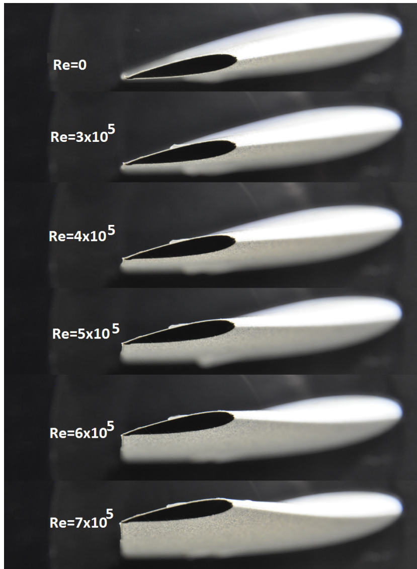
FIGURE 4.6 – Hydro-elastic response of the POM hydrofoil, \alpha = 10^\circ
