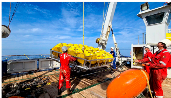
FIG. 7. Custom-made drag parachute being hoisted, with orange standard elliptic buoy on deck to the right.
