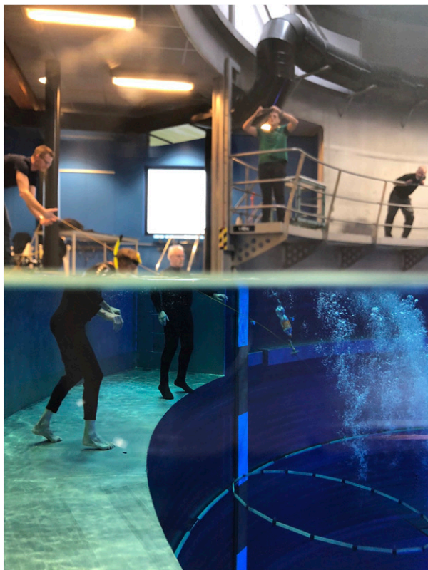
FIG. 6. Impression of testing the drag parachute using scale models in an 8-m-deep swimming pool. The large-ring steel model is in the lower-right corner, the drag parachute model just below the water surface to the left of the air-bubble columns.
