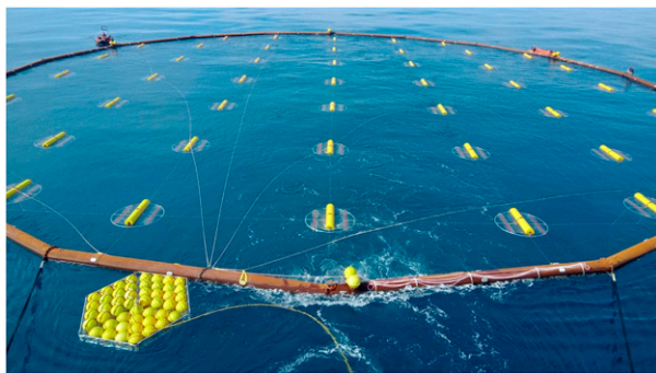
FIG. 1. The entire large-ring mooring array 3D-T in compacted form just before deployment. Visible are most of the 45 buoys on top of the small rings in which the mooring lines are folded up with T sensors. The small rings are attached to a steel cable network that is tensioned between the steel tubes and that is vaguely visible underwater. Outside the large ring, the drag parachute is attached in the front left. The drag parachute is connected to six white floating lines of which the nearest is attached in loops on the large-ring steel tube in the front. The two yellow balls contain glass spheres to underwater lift the acoustic release between them and to which the white line is attached, for removal of the drag parachute immediately after landing on the seafloor.
