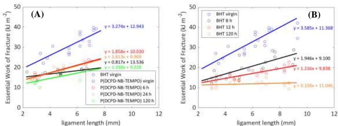
**Figure 4.** Impact of oxidation on fracture properties in (A) **P(DCPD-NB-TEMPO)** (left) and (B) **PDCPD-BHT** (right) at 60°C.
