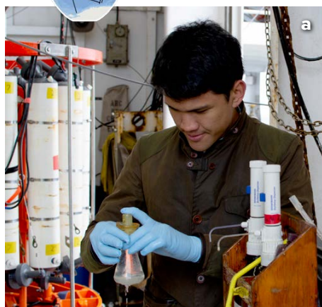
FIGURE 4. (a) Sampling for oxygen during GO-SHIP 108S on R/V Roger Revelle in 2016. Photo credit: Earle Wilson (b) A CTD/rosette package is launched during GO-SHIP 106S aboard R/V Thomas Thompson in 2019. Photo credit: Isa Rosso
