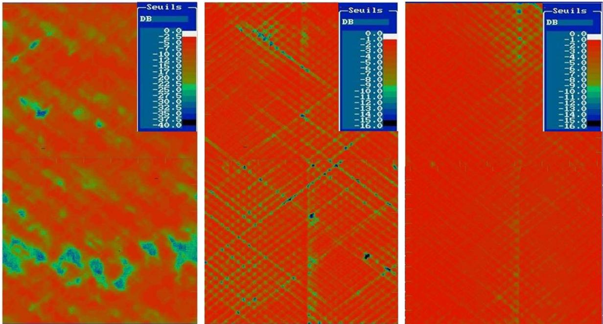
Figure 7. C-scan results (a) Epoxy 40 dB (b) PA12 16dB (c) PA6 16dB
