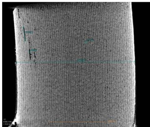
Figure 8. C-Scan Tomography, Carbon/polyamide 12 composite
