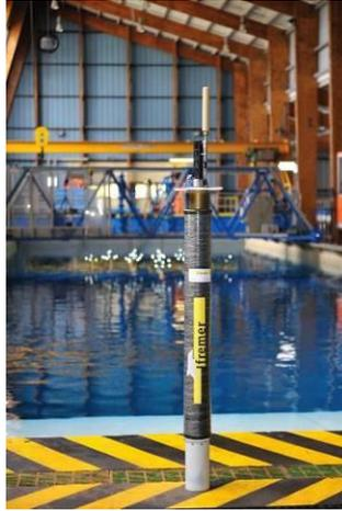
Figure 1: Deep Arvor carbon/epoxy profiler
