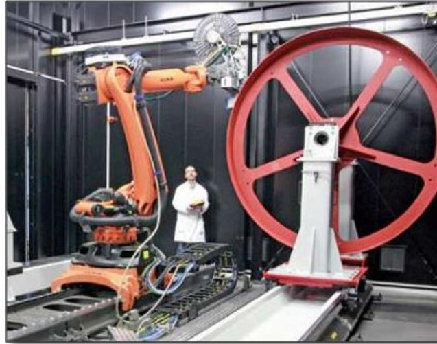
Figure 3. Laser Assisted Tape Placement machine
