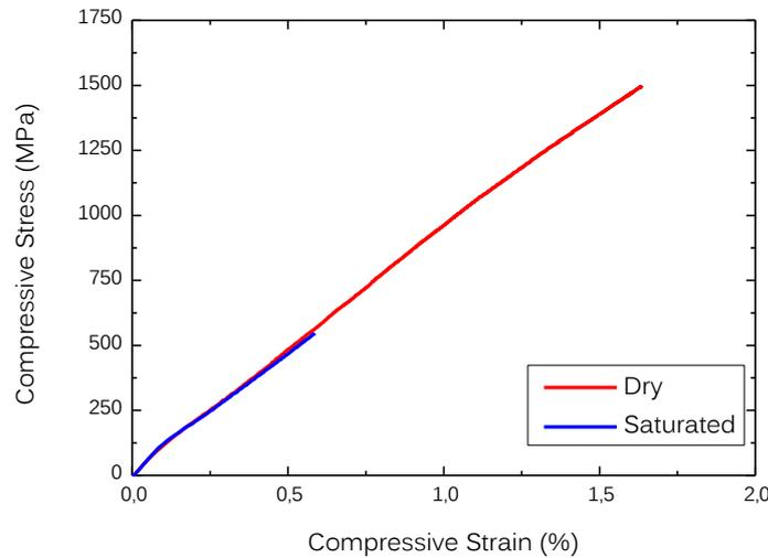
Figure 6. Compression stress-strain plots, before and after saturation
