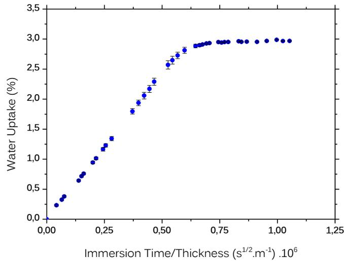
Figure 4. Diffusion kinetics, 40°C sea water carbon/polyamide 6, 2mm UD
