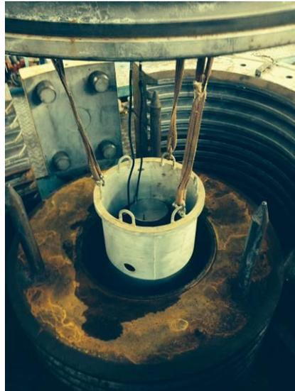
Figure 10. Cylinder being lowered into 2400 bar pressure vessel.
