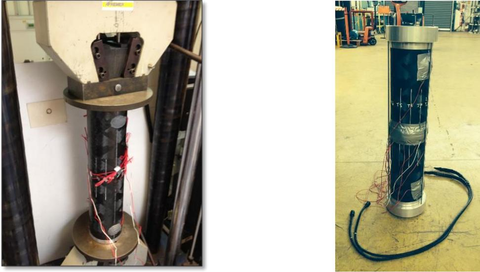
Figure 9. Cylinder samples, under axial compression and before pressure test.
