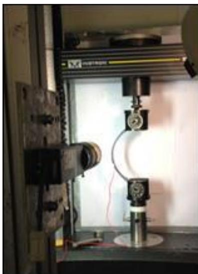
Figure 5. Compression test, strain gauged sample, camera to record shape change.
