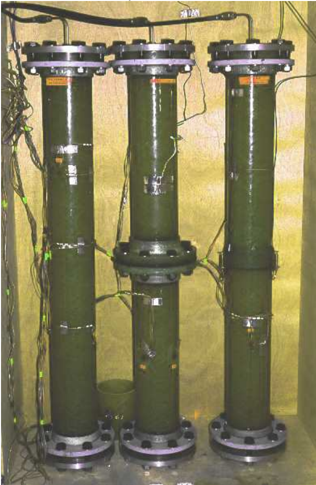
Photo 1. 20°C creep chamber with tubes of type A, B and C.
