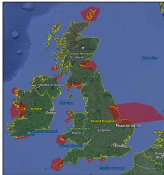
Figure 16 : Distribution of refinement polygons used in Polymesh
