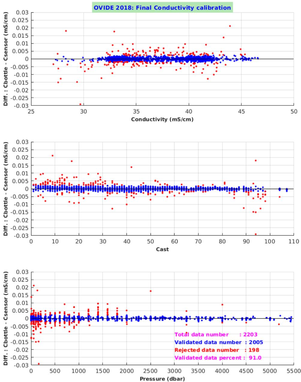
Figure 35: Final Conductivity calibration for OVIDE 2018.
