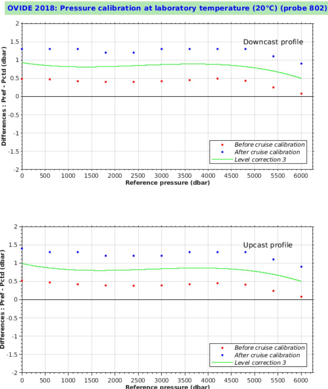
Figure 27: Pressure calibration at 20 °C
