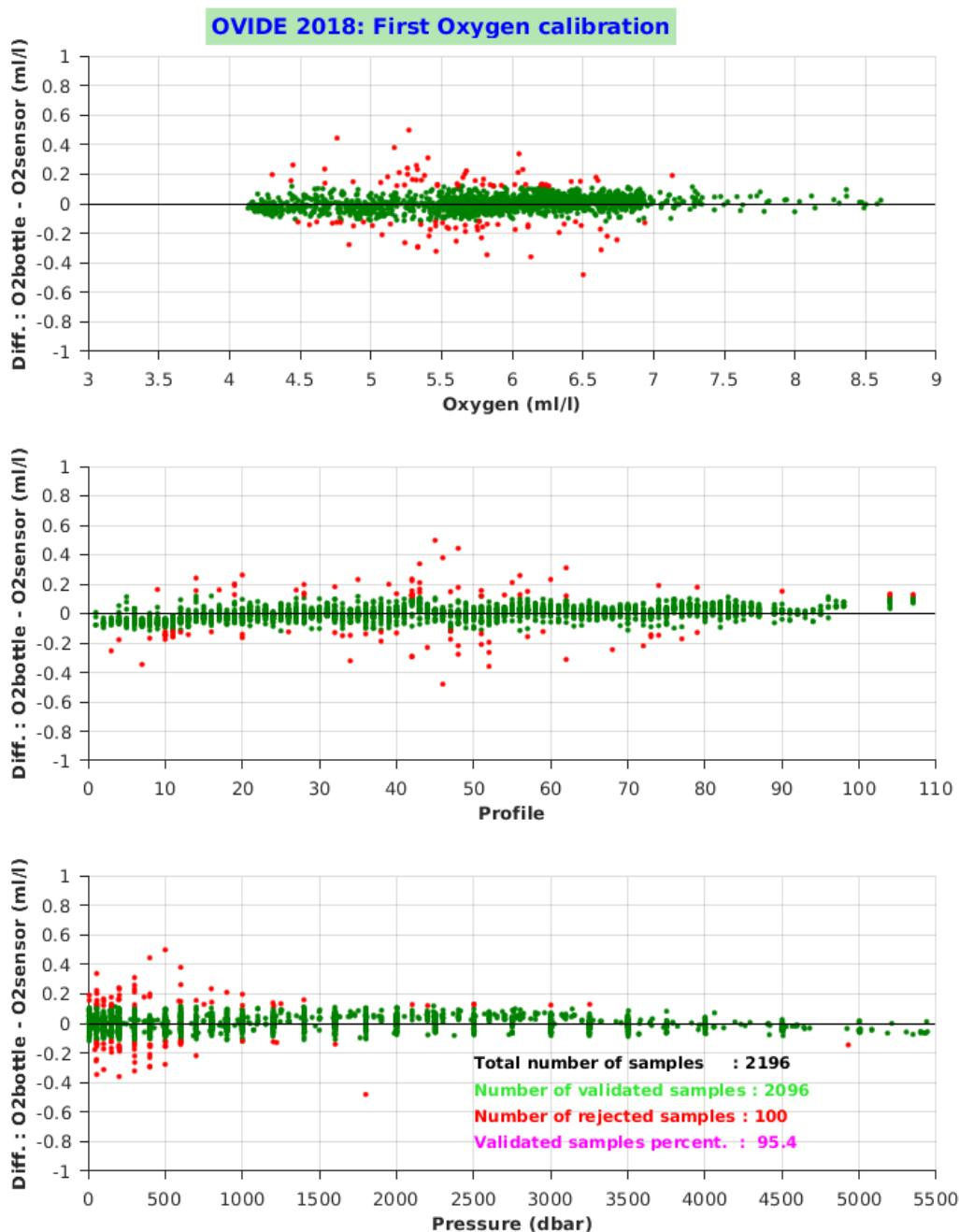
Figure 42: First Oxygen calibration.
