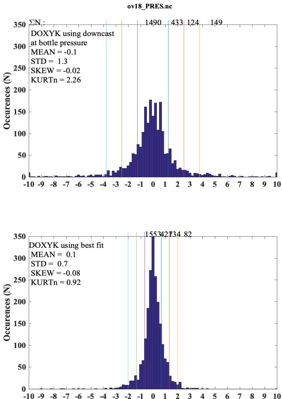
*Figure 51: Histogram of the oxygen difference between the chemical measurements flagged good and the probe data, in  $\mu\text{mol}.\text{kg}^{-1}$ , (a) using only downcast data at the bottle pressure level, and (b) using the best match between chemical and probe data by using either upcast data, downcast data at the bottle pressure level or downcast data at the bottle density level*
