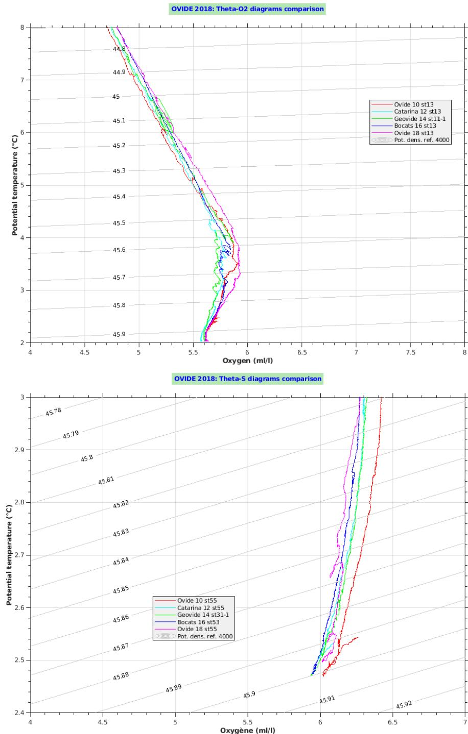
Figure 47: Theta-O<sub>2</sub> comparisons for stations made at (top) 40.333°N 12.223°W in Iberian Abyssal Plain, and (bottom) 54.762°N 26.125°W in Iceland Basin.
