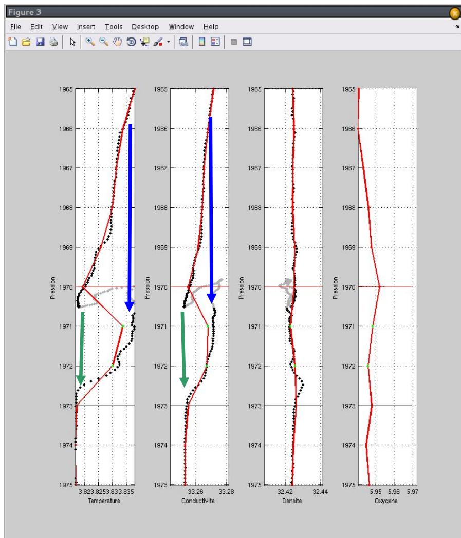
*Figure 50: Exemple of invalidation of density inversions.*
