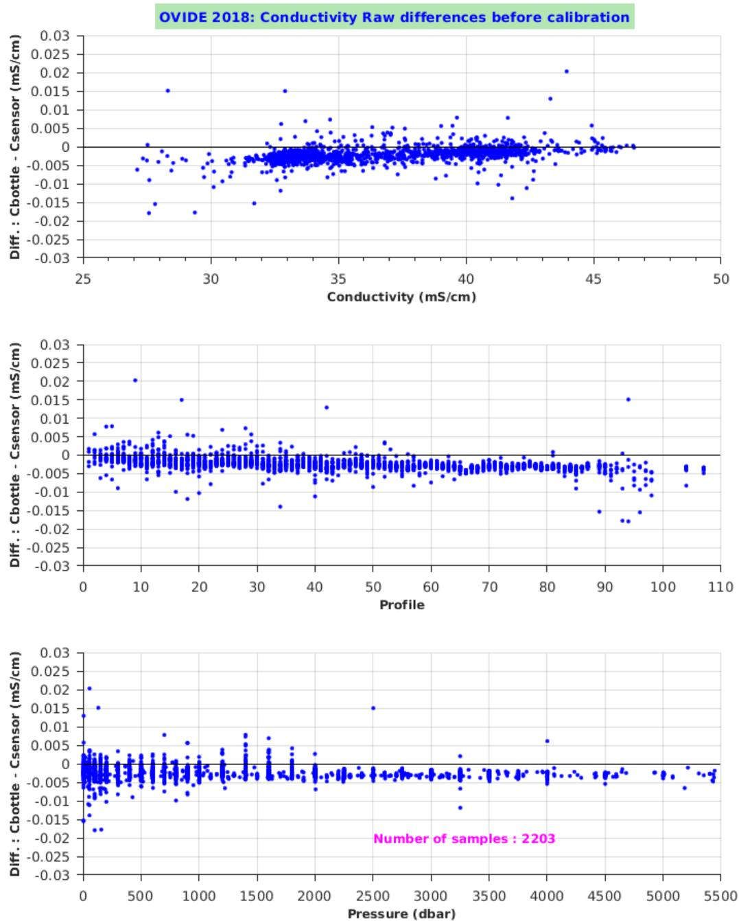
*Figure 33: Conductivity raw differences.*
