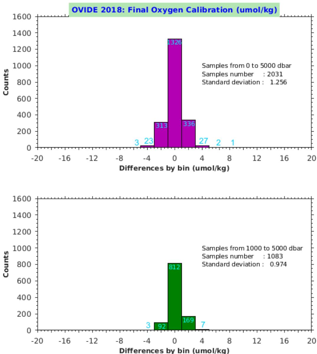
*Figure 45: Histogram of the Oxygen differences (umol/kg).*
