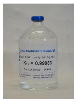
*Figure 20: Standard seawater*
