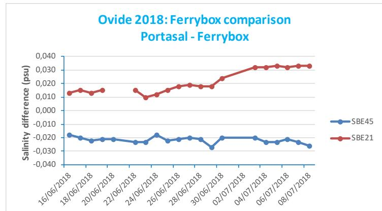
The plot on the right shows the differences between samples taken in the ferrybox circuit and analysed on board with a Metrohm titrino and the real time measurement of ferrybox.
