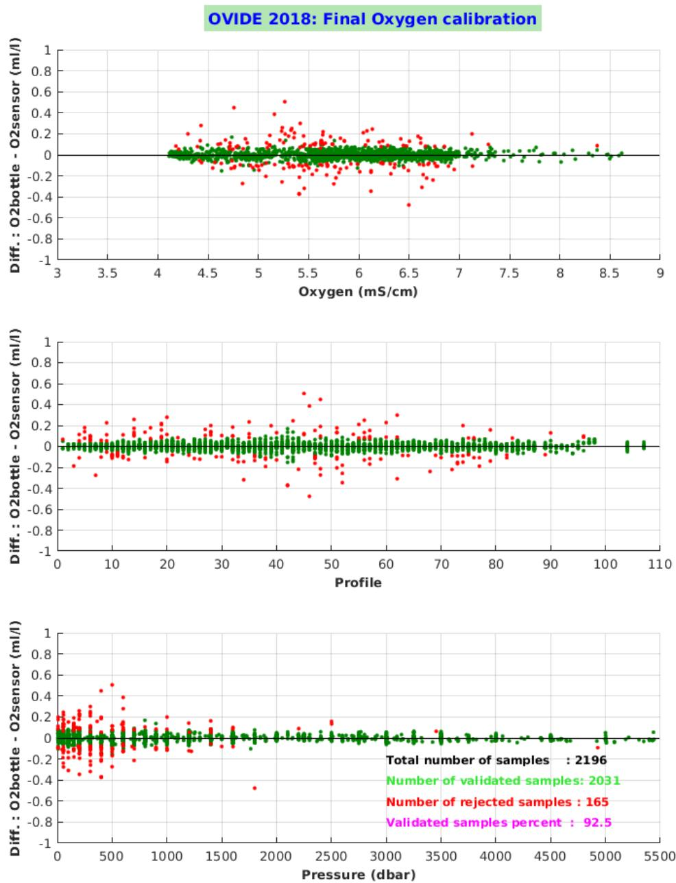
*Figure 43: Final Oxygen calibration.*
