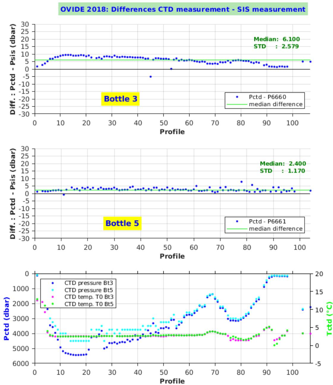
Figure 29: Comparison CTD pressure and SIS pressure
