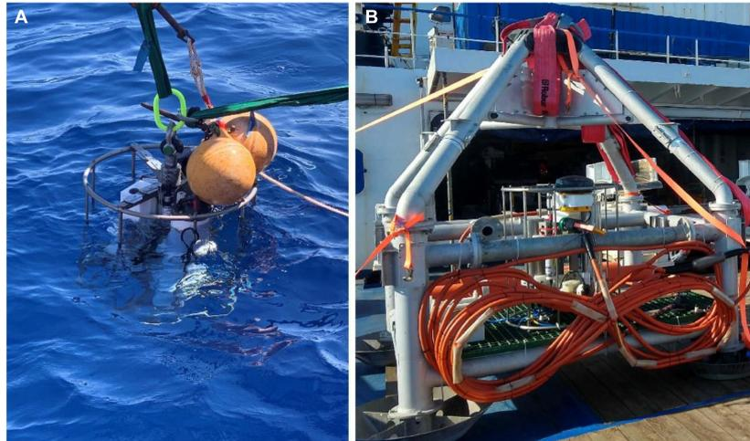
**FIGURE 3** | The EGIM (A) in a mooring line during the deployment in autonomous mode on ESTOC test site and (B) inside the pyramidal frame used at Western Ionian Sea with the electro-optical converter and the 50 m electro optical jumper for the connection to the submarine cable of the infrastructure.
