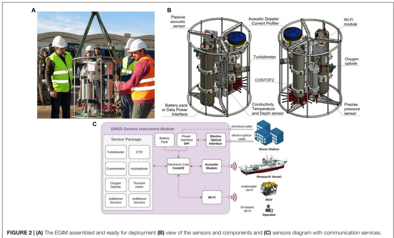
**FIGURE 2 | (A)** The EGIM assembled and ready for deployment **(B)** view of the sensors and components and **(C)** sensors diagram with communication services.
