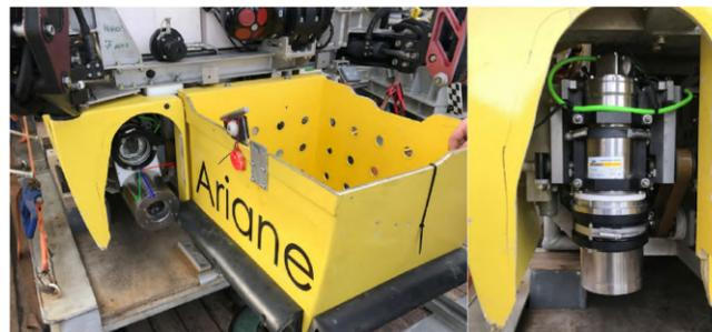
Fig. 1: Stereo setup of the two cameras on Ariane HROV from IFREMER [7], [8]. The upper is the RGB frame camera. The bottom is the pushbroom HS camera. The Z-axis is in the view direction, X-axis to the right and Y-axis pointing downwards. The cameras are mounted vertically having the y-axis as baseline between them.
