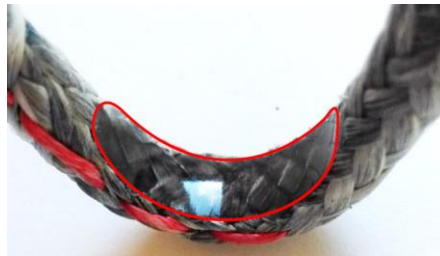
Figure 10. Visual observations of the contact surface between the textile axis and the ring of the pulley.
