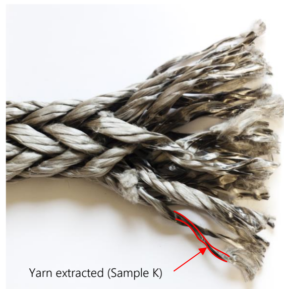
Figure 2.b. The different scales of the Dyneema™ SK78 braided rope with a diameter of 22mm, coating and a MBL of 500kN (Sample K in red)
