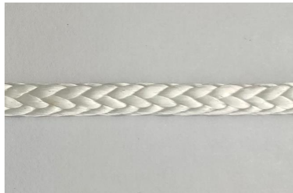
Figure 3. b. Uncoated HMPE fiber rope, 4mm diameter
