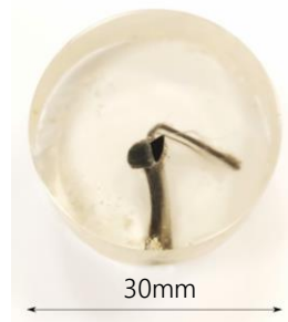
Figure 8. Sample K cast in resin ready for digital microscope observations
