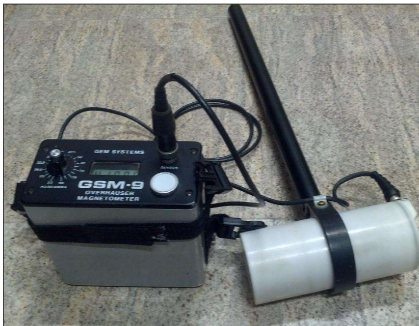
Figure 3.2. Magnetometer GSM-8 used to acquire magnetic data during this Ph.D. Thesis.
