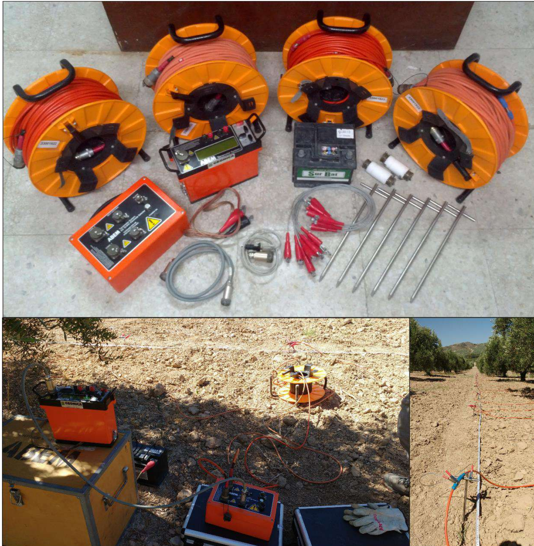
Figure 3.3. Terrameter SAS 4000 used to obtain the ERT profiles of this Ph.D. Thesis. Lower photos show the dispositive carried out on the field.
