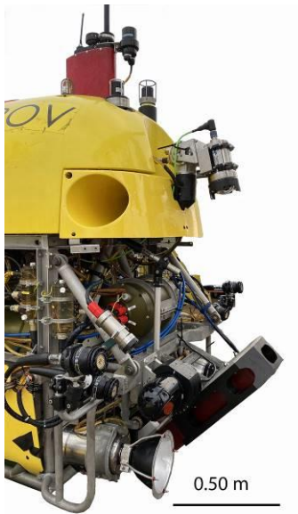
Figure 1. Image of Ariane H-ROV with the Kongsberg EM2040 Multibeam Echosounder installed with a 45° angle.
