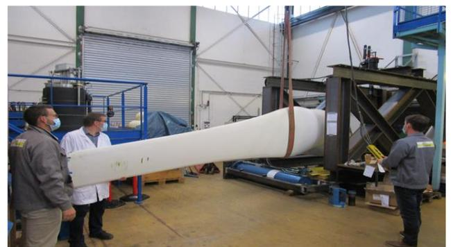
Fig.12. Blade installation on the test frame.
