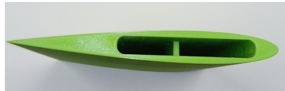
Figure 5: 3D printing NACA 0012 with fairing system.
