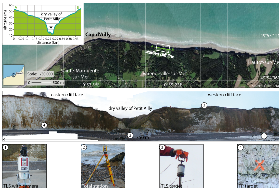
Figure 1. Panorama and aerial photography of Petit Ailly cliff (Varengeville-sur-Mer) and instrumentation used for the TLS survey (2016-01-28) (modified from Letortu et al. (2018)).
