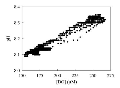
**Supplementary Figure 2:** Relationship of dissolved oxygen (DO) concentrations ( $\mu$ M) and pH measured simultaneously in October 2021 with a WiMo Plus multiparameter probe (*NKE Instrumentation*) by profiling in the water column of the continental shelf off the Gironde (13 profiles). The significance of the correlation was confirmed by a Spearman rank correlation (p<0.01, n=2351).
