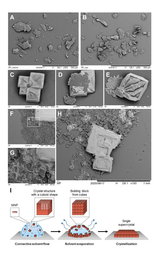
Figure 5. Representative SEM images of microplastics in the 20–60  $\mu m$  fraction produced in this study and their spontaneous self-assembly into crystal superstructures through slow solvent
