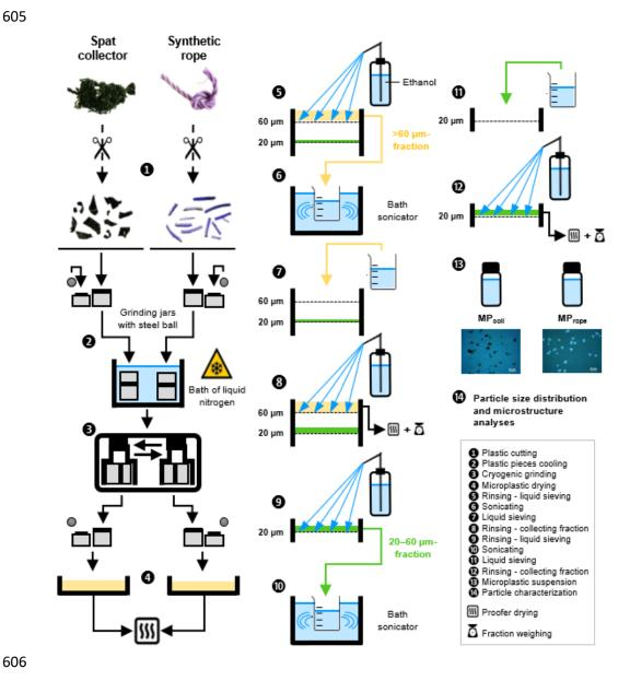
Figure 2. Synthetic diagram of the microplastic production method tested.
