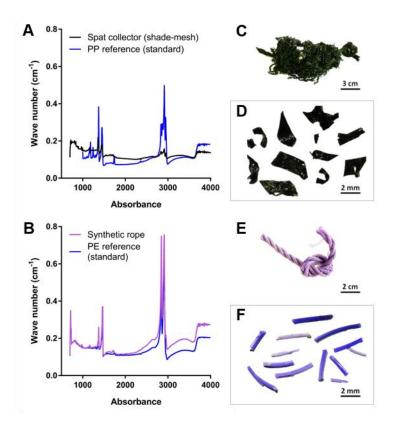
**Figure 1.** Polymer identification in two plastic pearl farming gear types by FTIR. Polypropylene (PP) for the spat collector (A) and polyethylene (PE) for the synthetic rope (B). Photographs show the spat collector (C) and synthetic rope (E) and their associated plastic pieces (D and F, respectively) used for MP production. Spectra of particles produced were identical to those of plastic gears, hence not added here. Adapted from Gardon et al. (2020a).
