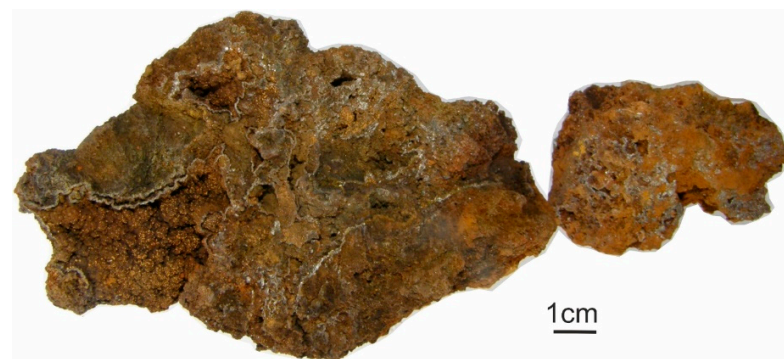
Figure 15. A general view of sulfide samples from st. 373. Porous massive sulfides oxidized from the surface.
