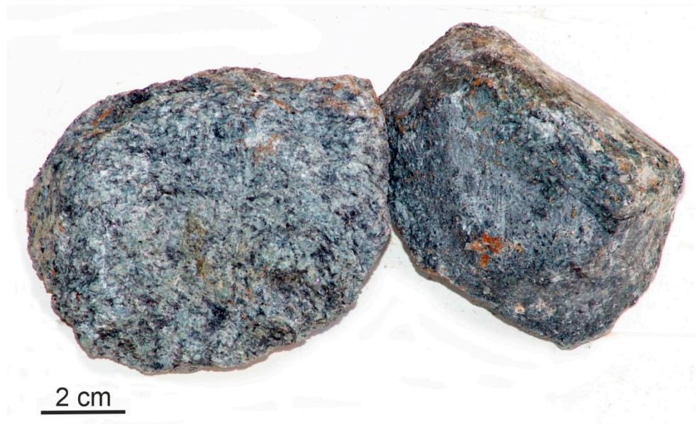
Figure 10. A general view of sample 242 with vein-disseminated mineralization.
