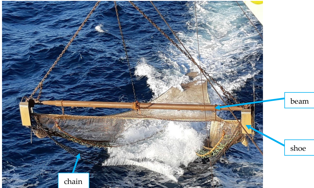
Figure I.2. Example of a beam trawl (used in the Dutch survey) with its elements indicated.
