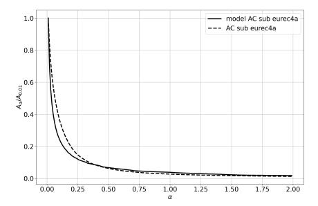
Figure 10. Intensity of eddy boundaries: comparison between data (dashed line) and model (continuous line). The ordinate axis represents the normalized boundary. The abscissa axis is showing the value taken by  $\alpha$ .
