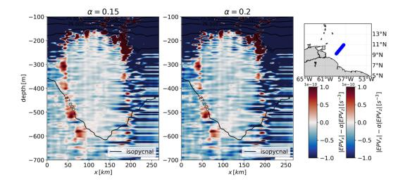
Figure 4. The  $\alpha$ - criterion to define the eddy boundary for different thresholds:  $\alpha = 0.15$  and  $\alpha = 0.2$ . This criterion (in dark red) surrounds the core and extends from 10km to 50km. Note that this limit coincides with the inflection points of the isopycnals (see the theoretical part developed in the main text in section 5). The small geographical map shows where the oceanic eddy was sampled.
