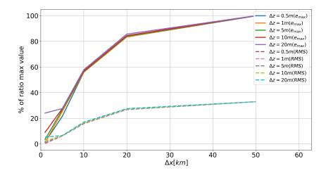
**Figure 9.** Maximum RMS and maximum error, in percentage of the ratio maximum value, as a function of horizontal resolution. Curves are plotted for various value of  $\Delta z$ .
