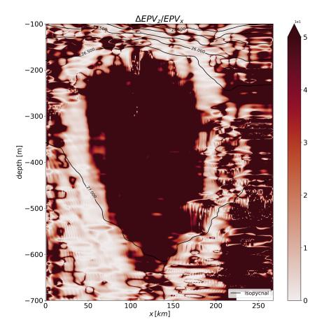
Figure 11. Vertical section representing the modulus of the ratio between  $\Delta EPV_z$  and  $EPV_x$ ; Colors have been saturated in order to obtain an homogeneous core. The clear boundary represents the region where the baroclinic term  $EPV_x$  has a non negligible value compare to  $\Delta EPV_z$ .
