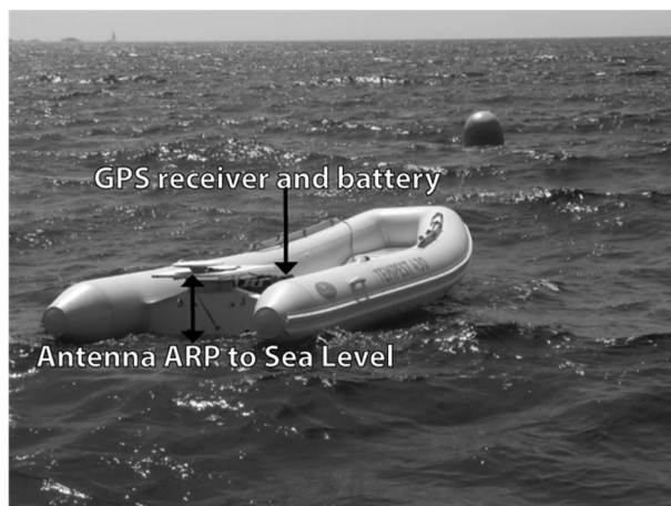
Figure 1. Zodiac boat used as GNSS-based sea level measurement system since 2012. GNSS receiver is on-board and connected to the antenna located at the rear.
