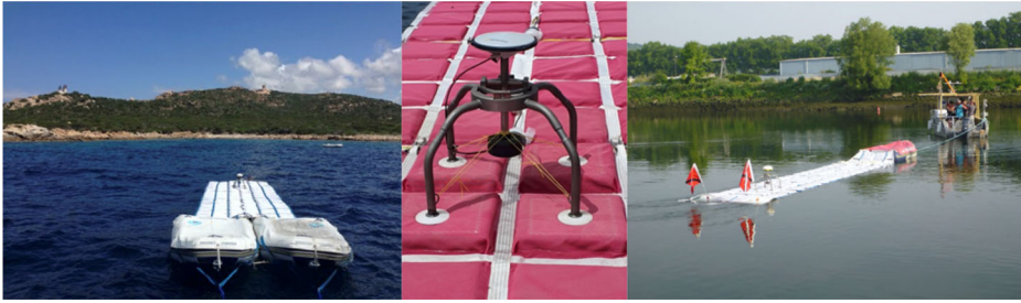
Figure 2. Photos of CalNaGeo. Left: for offshore use (open ocean; two inflatable boats) during this experiment (the GNSS-Zodiac can be seen on the right in the background and the lighthouse, where the reference receiver is, on the left in the background). Right: for inshore use (coastal ocean, lakes, rivers; one inflatable boat) during a campaign on the Seine river, France in June 2017. Middle: zoom on the gimbal system (photo from another experiment).
