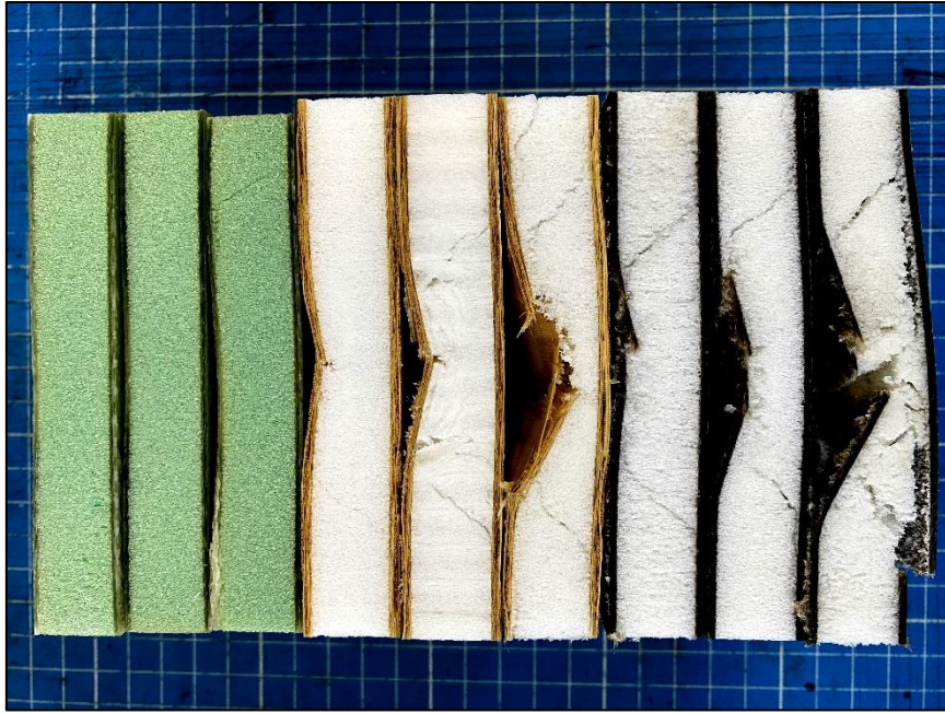
Figure 9 - Section of coupons of Glass/PVC, Bamboo/PET and Flax/PET coupons impacted at (from left to right) 21J, 43J and 82J.
