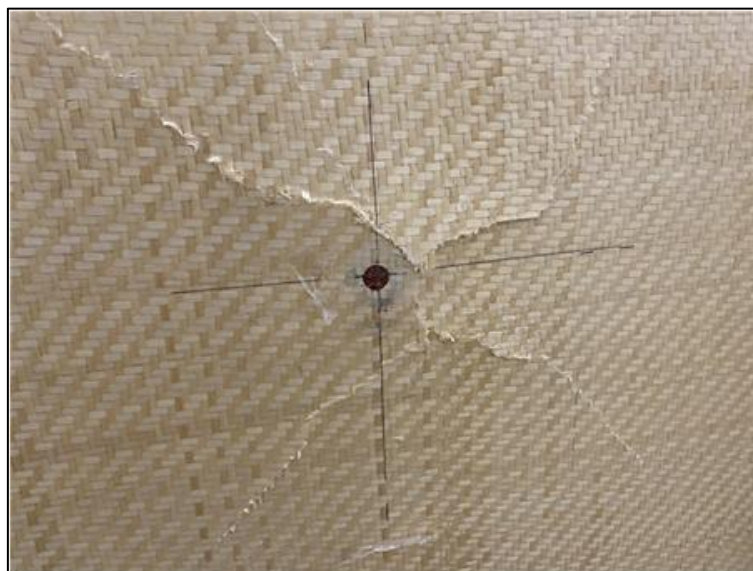
Figure 11. Images of panels after 1225J slamming impacts
