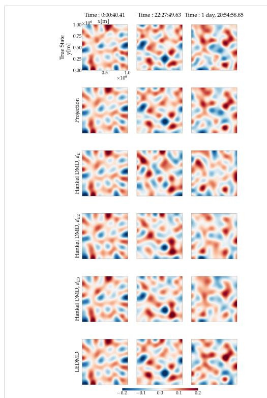
**Figure 5.** Forecasted Shallow Water fields with respect to the projections and true states. First row: Ground truth; Second row: Projection from the EOF basis; Third, fourth and fifth rows: Hankel-DMD based algorithms with the Hankel matrix features dimension  $d_{E1} = 700$ ,  $d_{E2} = 10\,000$  and  $d_{E3} = 20\,000$  respectively; Sixth row: Proposed EEKF model with  $d_E = d_{E1} = 700$ . The error time series of these experiment are provided in figure 6.
