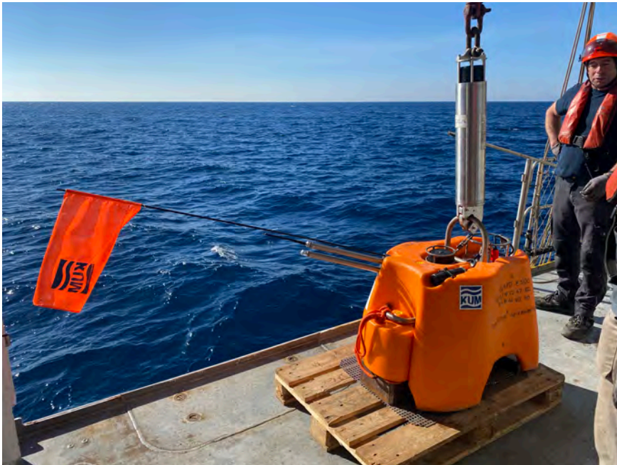
Figure 10: deployment of Nammu ocean bottom seismometer.
