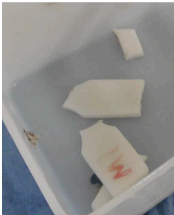
Fig. 5. PLA matrix tensile specimen pieces after eight months' immersion in seawater at 40 °C.
