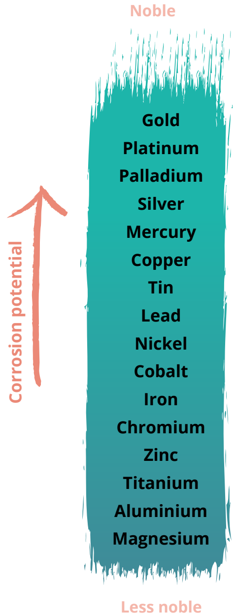
Fig. 1 Diagram showing the classification of different metals according to their corrosion potential in a seawater environment. Based on the definition of corrosion given by AFICPAR 3 .
