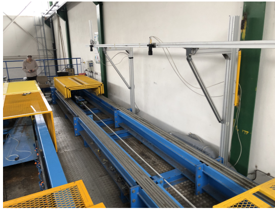
Figure 2: Rope tensile testing set-up equipped with cameras for strain measurements.
