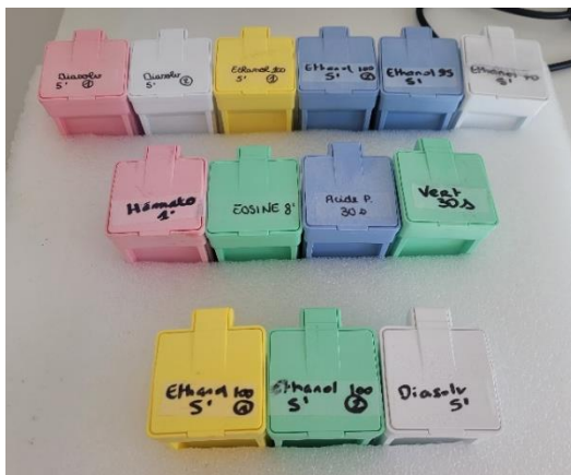
Figure 20. Plastic tanks noted with the solution they are filled and the bath times.
