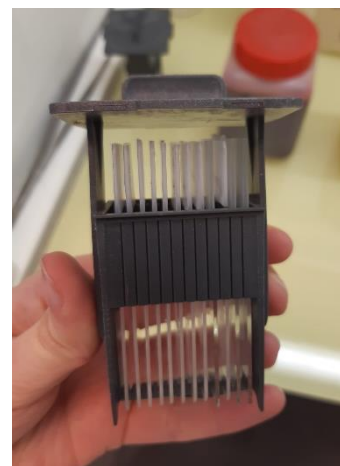
Figure 3. Slides staining holder
