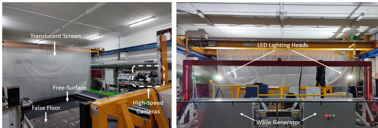
Figure 1. Boulogne-sur-Mer experimental campaign setup. On the left: Experimental setup on the cameras side. On the right: Setup, behind the translucent screen
