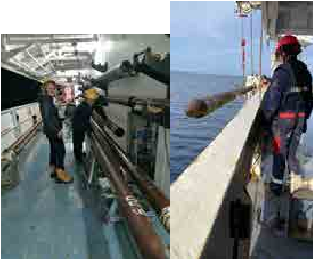
Figure 22: Left panel, Activation of THP sensors before corer launch. Right panel, launching of the corer equipped with the sensors.
