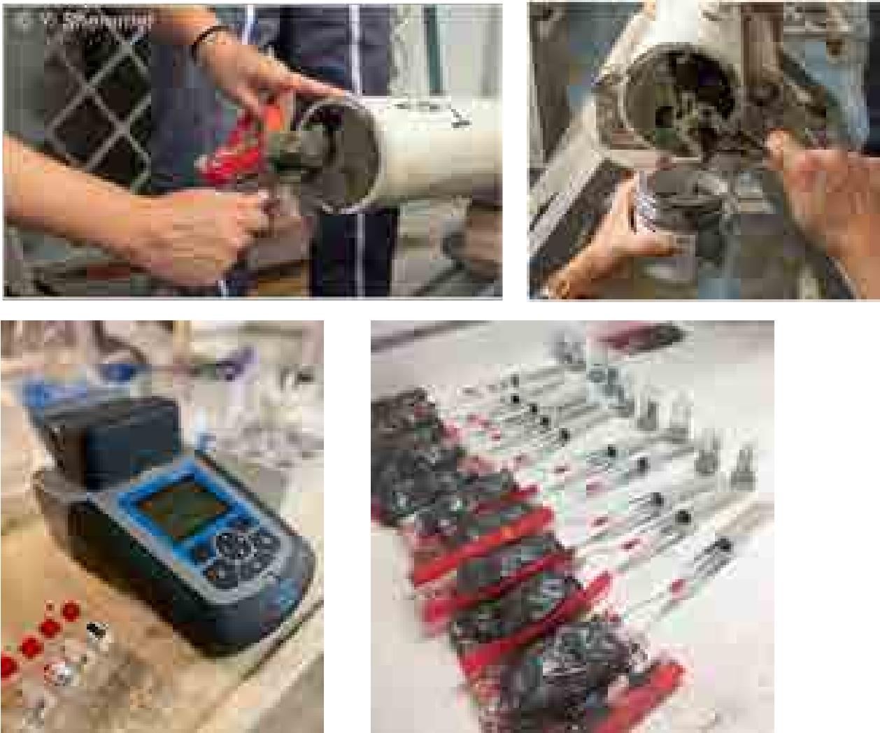
Figure 29: Onboard sulphate analyses. Sulphate and methane concentration were measured on pore fluids systematically at each core base.
