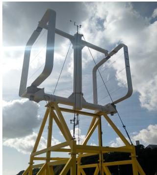
Figure 1: The 10kW WindQuest VAWT in the Ifremer *in situ* test station of Brest
