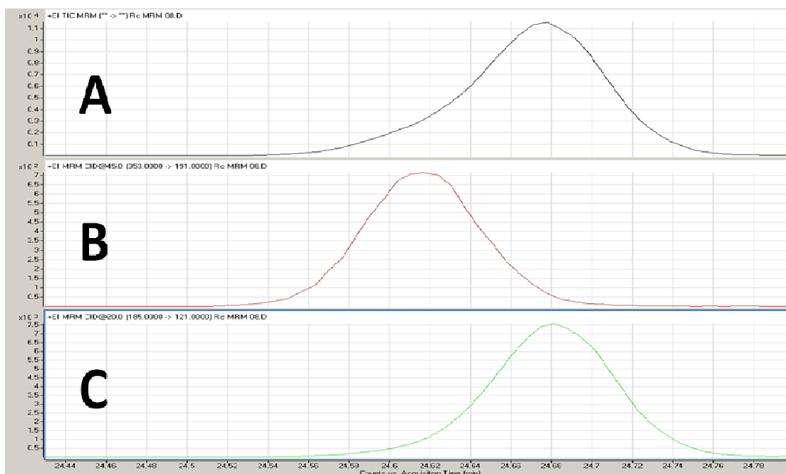
Figure 6.2. Coelution of oxychlordane and heptachlor epoxide. From top to bottom, A) total ion chromatogram, B) extracted reaction chromatogram for heptachlor epoxide and C) extracted reaction chromatogram for oxychlordane.
