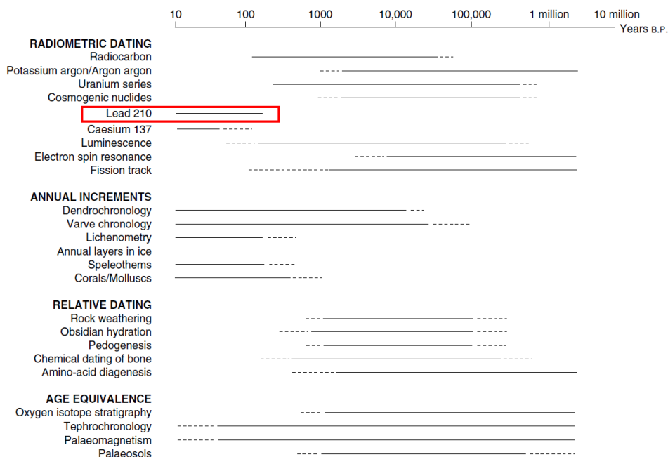
Figure 23. Temporal ranges for different dating techniques. Framed in red is the ^{210}\text{Pb} method chosen here for Anthropocene detection in marine sediments. Source: Walker, [2005].
