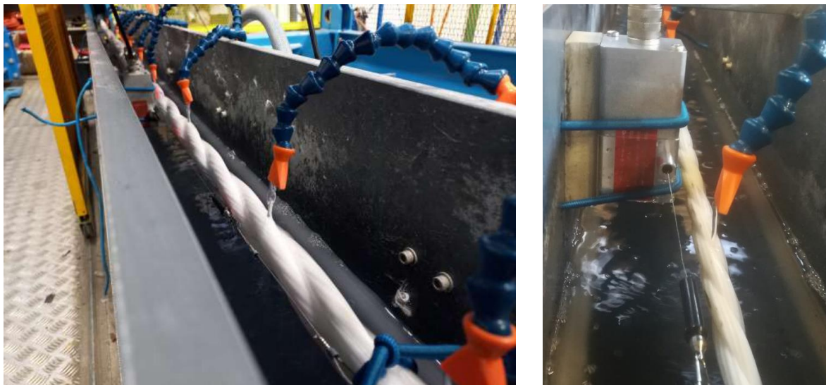
Figure 1: 30 ton test bench with sprinklers and tensioned wire sensor
