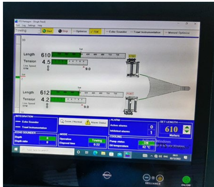
Fig 4.2 Screen for the RappHydema autotrawl system showing tension on the winches of 4.2 tons during one of the comparative hauls.
