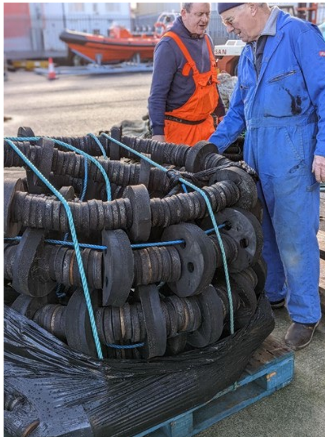
Fig 2.2.2 Groundgear layout for the revised survey trawl.
