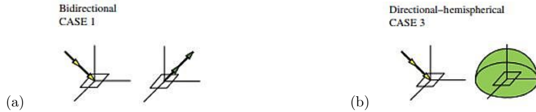
Figure 3.1: Measurements geometries from (Schaepman-Strub et al. 2006) (a) CASE 1 Bi-directional, (b) CASE 3 Directional-hemispherical.
