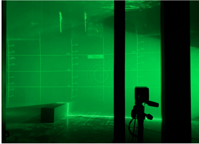
Figure 3: PIV setup with the camera in foreground and the laser sheet illuminating the square cylinder. The resistive wave probes are passing through the free-surface where a wave-trough is visible on top of the cylinder.
