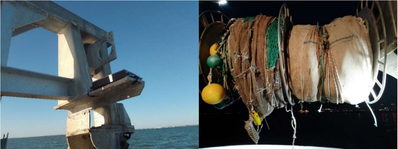
Figure 10. MOANA system from ZebraTech tested as part of the DELMOGES project (left: multi-function box, right: probe)
