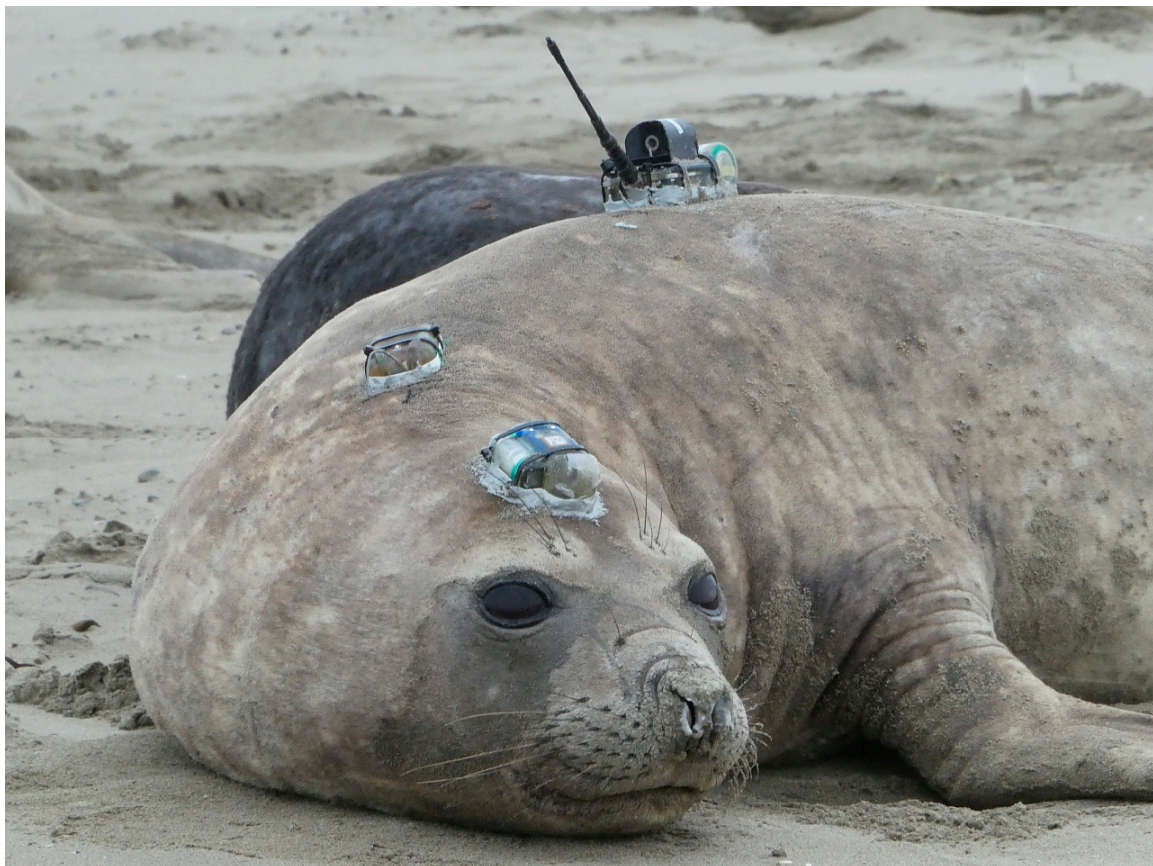
Figure 2. A female SES with three biologging devices glued: a head-mounted DTAG-4, a back-mounted CTD-SRDL, and a neck-mounted SPOT. The main characteristics of the devices are listed in Table 2.
